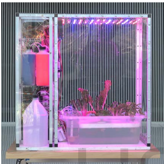
Fig. 1: OpenAg™ Food Computer (FC) has an improved software controller and additional sensor and actuation capabilities.
